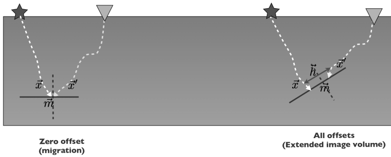
Figure 1: Subsurface image volume as a function of the source and receiver subsurface coordinates \vec{x} and \vec{x}' , where the stars and triangles stand for the sources and receivers respectively. The vectors \vec{m} and \vec{h} represent the full multidimensional subsurface midpoint and offset coordinates defined as in equation 2.
