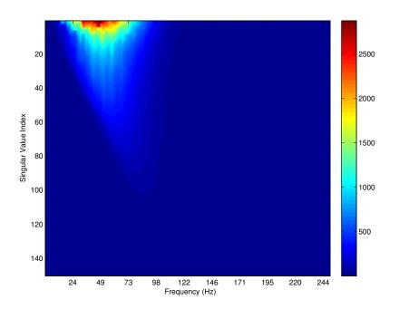
Figure 3: Singular values for data matrices as a function of the frequency. As expected, the largest singular values are concentrated within the seismic band.
