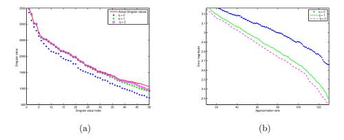
Figure 10: Decay of the singular values for a single frequency at 100 Hz for  $n_r = n_s =$  150. (a) Approximation of the singular values, and (b) the behavior of the spectral approximation error.
