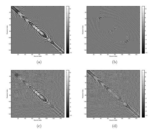
Figure 13: Low-rank factorization of a frequency slice at frequency of 100 Hz and  $n_s = n_r = 150$ . (a) HSS approximation (relative spectral norm = 0.22), (b) the difference between the HSS approximation and the original data matrix, (c) SVD approximation of the same frequency slice (relative spectral norm = 0.43) and (d) the difference of the SVD approximation with the original data matrix.
