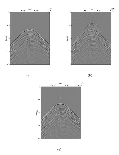
Figure 4: Adaptive versus non-adaptive rank selection. (a) prediction of multiples with the full data matrix, (b) prediction with the low-rank factorization for  $\delta = 1/12$ , and (c) the prediction with adaptive rank selection.
