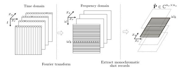
Figure 1: Extraction of monochromatic wavefield matrices, by transforming the data from the time domain into the frequency domain via the Fourier transform. Then, for each frequency component a data matrix  $\hat{\mathbf{P}} \in \mathbb{C}^{n_r \times n_s}$  is extracted (adapted from Dedem (2002)).
