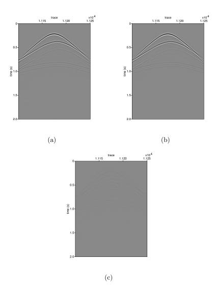
Figure 16: EPSI results from the synthetic dataset. (a) Estimated Green's function using the full dataset, (b) estimated Green's function with low-rank approximation for  $\delta = 1/12$ , and (c) difference plot.
