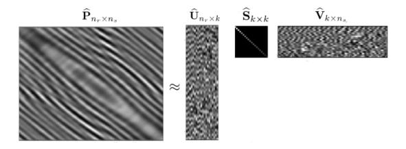
Figure 2: Matrix factorization by SVD for a frequency slice  $\widehat{\mathbf{P}} \in \mathbb{C}^{n_r \times n_s}$  on the left, and its SVD decompositions on the right. The matrix  $\widehat{\mathbf{U}}_{n_r \times k}$  and  $\widehat{\mathbf{V}}_{k \times n_s}^*$  contain the left and right singular vectors of  $\widehat{\mathbf{P}}$ , respectively. The diagonal matrix  $\widehat{\mathbf{S}}_{k \times k}$  contains the singular values of  $\widehat{\mathbf{P}}$  on its diagonal.
