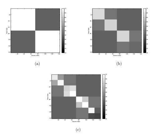
Figure 12: HSS partitioning of a frequency slice at 100 Hz. The grey scales correspond to the rank of the sub matrix (white is high-rank and black is low-rank) (a) First level of HSS partitioning; (b) second level; (c) third level.
