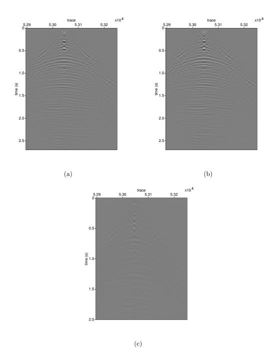
Figure 19: EPSI result for the gulf of Suez dataset. (a) Estimated Green's function with the full data matrix, (b) estimated Green's function for low-rank approximation for  $\delta = 1/12$ , and (c) difference plot.
