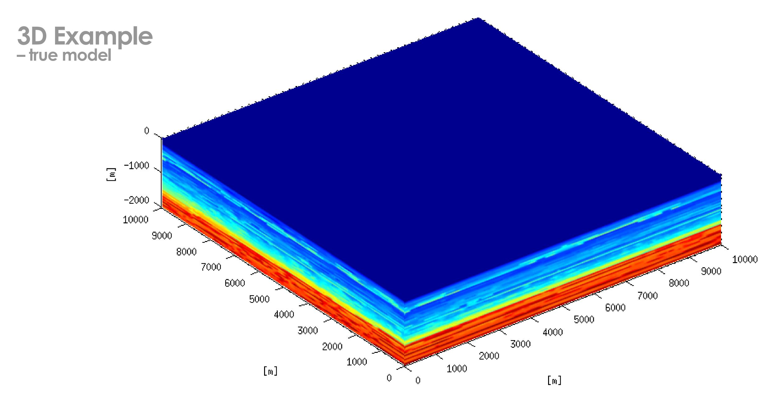
10 x 10 x 2 km, 5 Hz, 27-point discretization, ~1e7 grid points, source at [0,0,0]
